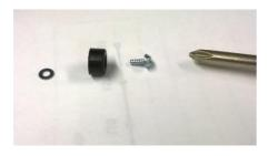
• Note: Install the 4 replacement feet with the washer against the printer housing or bracket. Insert screw from
